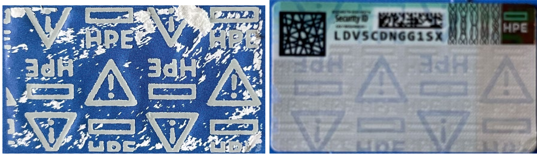
Figure 9: Adhesive left behind on product (left) and signs of tampering on label (right) on current label
