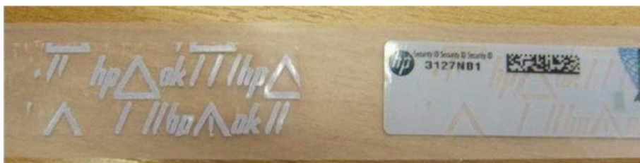
Figure 12: Adhesive left behind on product (left) and signs of tampering on label (right) on previous label
