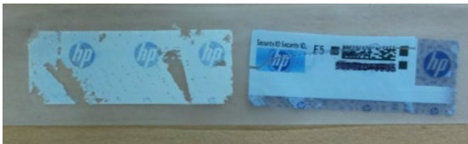
Figure 11: Adhesive left behind on product (left) and signs of tampering on previous label
