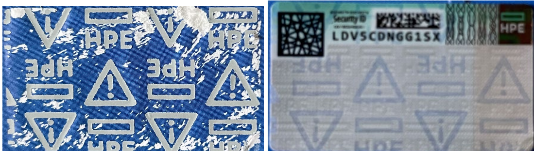
Figure 13: Adhesive left behind on product (left) and signs of tampering on label (right) on current label
