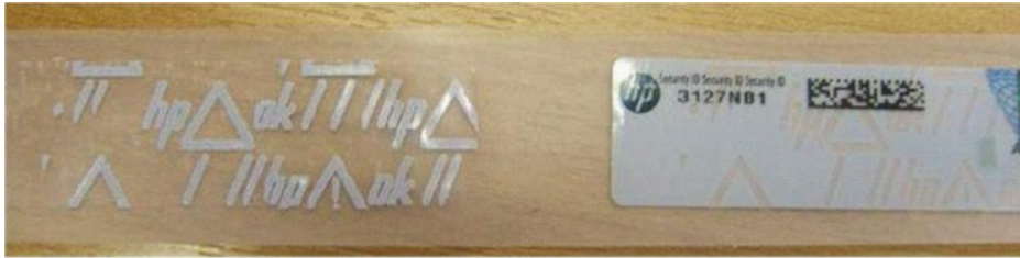
Figure 17: Adhesive left behind on product (left) and signs of tampering on label (right) on previous label
