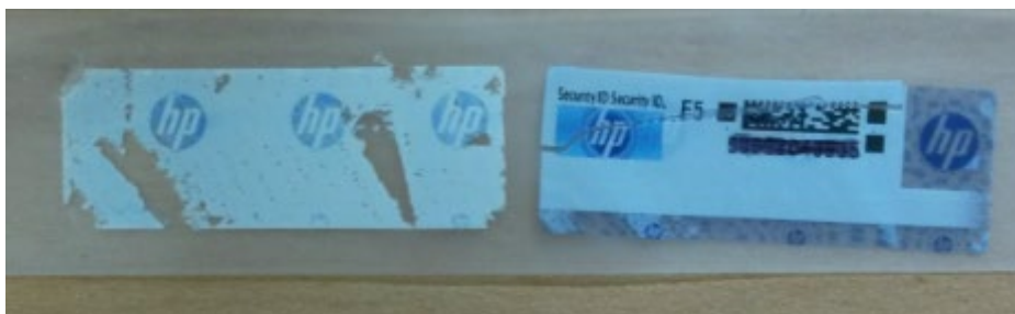
Figure 16: Adhesive left behind on product (left) and signs of tampering on label (right) on previous label
